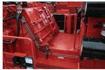
Extended Maintenance Platform
