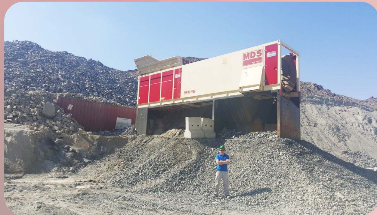
M615 stationary trommel 6m (20ft) x 1.5m (5ft) set up beside overburden in Oman quarry producing 4 products
