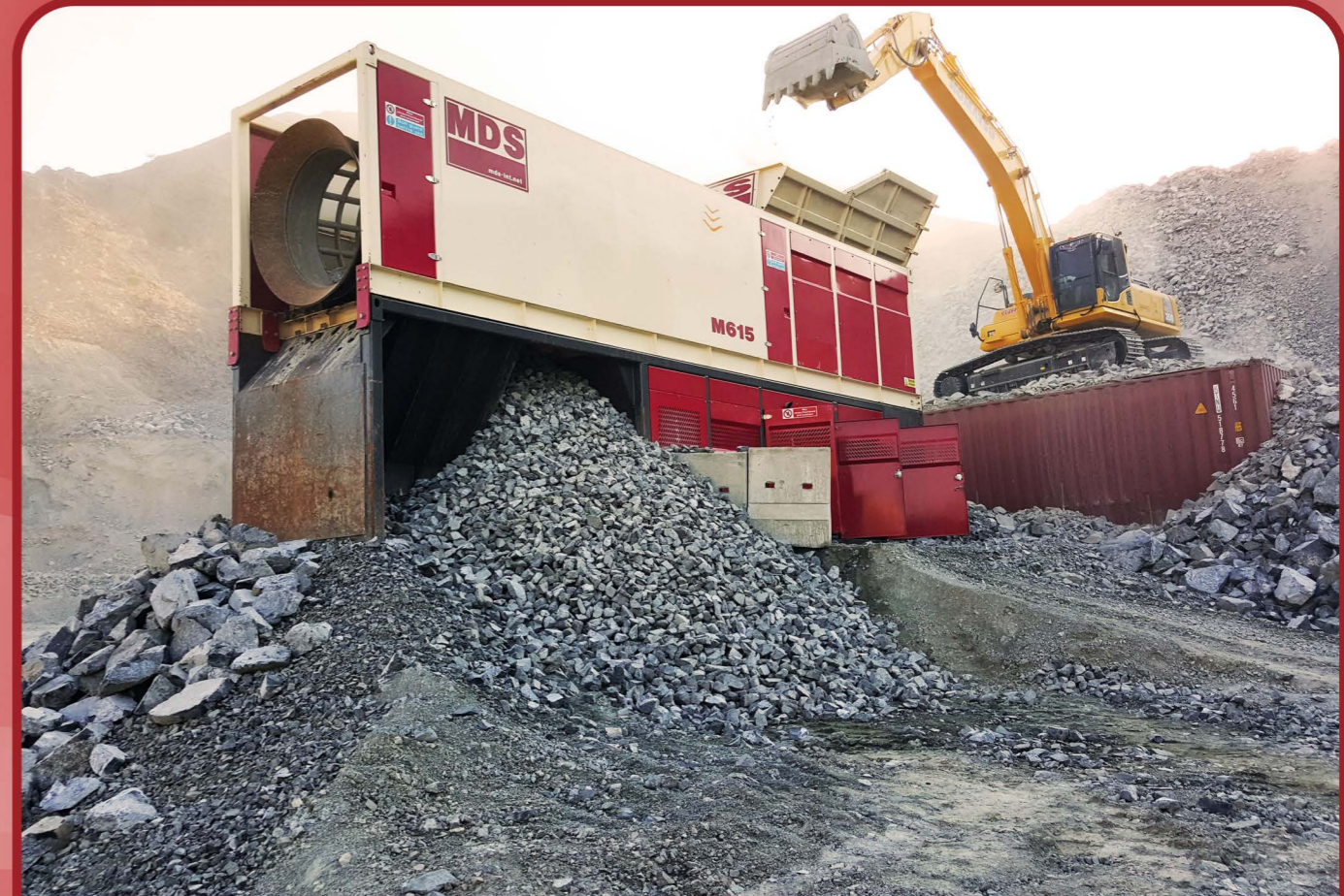
M615 mid product producing 150-250 mm (6"-10") material for customer
