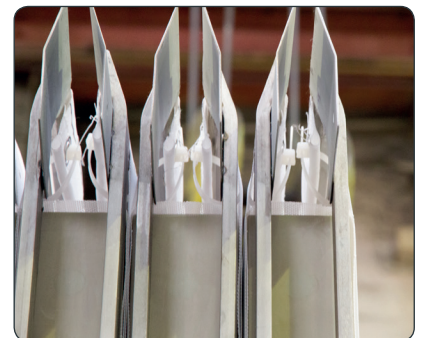
Cake discharge device in stainless steel
