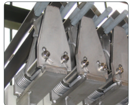
Cake discharge device in stainless steel
