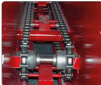
Plate transport mechanism with revolving chain
