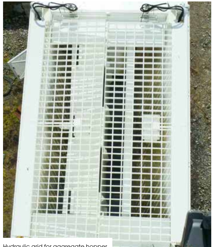
Hydraulic grid for aggregate hopper
