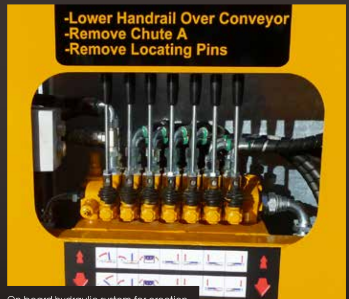
On board hydraulic system for erection
