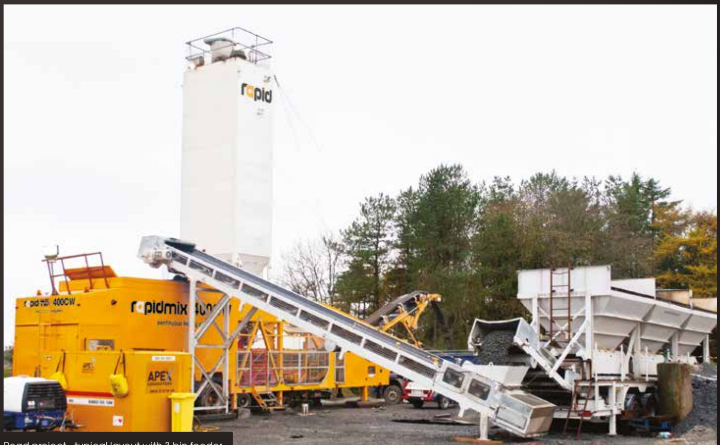
Road project - typical layout with 3 bin feeder
