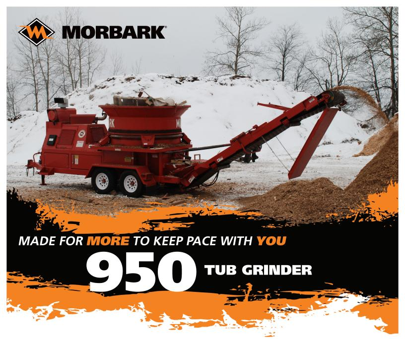
Compact and easy-to-haul, the **Morbark 950 Tub Grinder** is ideal for converting yard and wood waste, pallets and other mixed woody feedstocks into saleable products. The 950 tub grinder is equipped with a proven drive line protection system that protects against catastrophic damage from contaminants.
