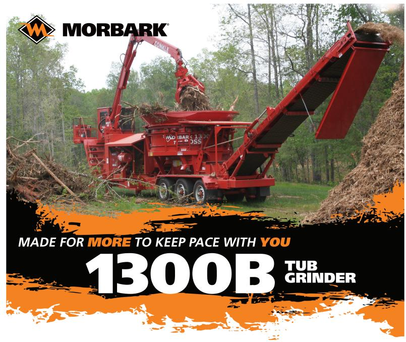
The **Morbark 1300B Tub Grinder** combines heavy-duty construction with the latest technology, including the Morbark Integrated Control System, which allows you to monitor critical machine parameters. With a full breakaway torque limiter system, hydraulic augers and a laser-cut hammer mill, the 1300B tub grinder is the most popular grinder on the market. The optional track undercarriage makes it easy to bring the grinder right to the material.
