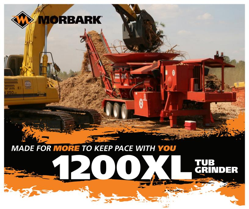
The **Morbark 1200XL Tub Grinder** is a mid-sized grinder that features the Morbark Integrated Control System for the ultimate in diagnostics; dual hydraulic tub drive motors for increased torque and greater efficiency; hydraulic augers for quick removal of product from beneath the mill; laser-cut, factory-balanced hammermills with forged hammers for unsurpassed durability and smooth operation; and tub tilt for easy access to grates and anvil for routine maintenance.
